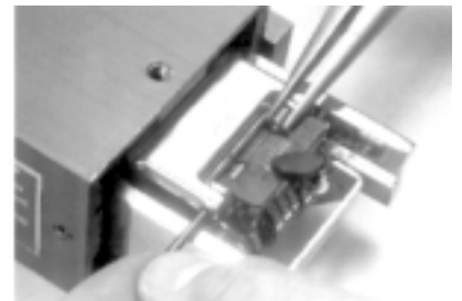
Installing the new springs
