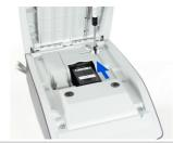
Keep fingers away from the ink cartridge while it is moving to the replacement position.
