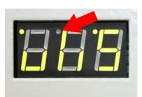
Middle dot shows correct function of sensor of counter. To find out if sensor of counter works correctly, outshine it by piece of paper. If everything ok, the middle dot stops shining. Once the paper has been removed, the dot starts shining again. Sensor is placed in the middle between left and middle feeding wheel table.
