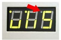
Right dot shows correct function of sensor of feeding table. To find out if the sensor works correctly, we outshine it by piece of paper. If the sensor is ok, the right dot stops shining.
