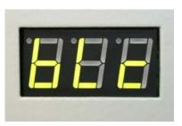
Symbol "blc" appears if rollers are blocked and the motor is overloaded.
