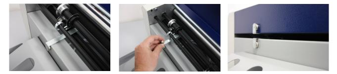
To remove the perforating wheels or the creasing wheel, it is necessary to remove the shaft with the strippers first and then remove the shaft with the perforating wheels. Remove the shaft by holding the bearing (39) and pull it over the spring into the terminal position. Then push the whole shaft back including the bearing that you continue to push into the terminal position, and remove the shaft from the machine as per the figure.
