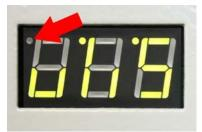
Left dot shows correct function of sensor, which defines revolutions of motor. Slowly move the pulley. If everything is ok, left dot stops shining always when sensor is not blocked by screen.
